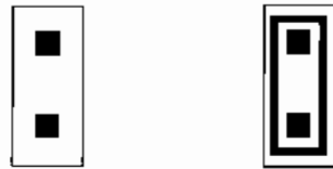
Figure B-2: Representation of disabled (left) and enabled (right) jumpers.
